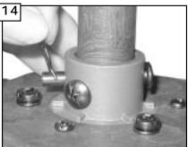
Install cotter pin into cross pin.
